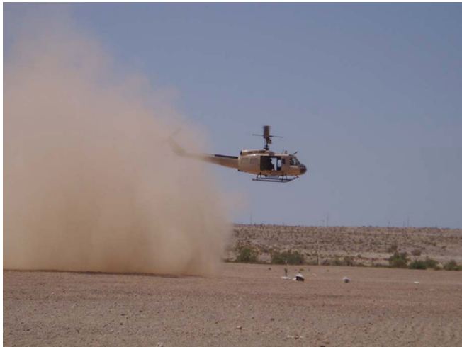
Fig. 1. The test aircraft creating dust emissions in the designated flight path at Site 2, Yuma Proving Ground.
