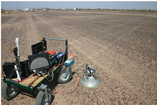
Fig. 5. The DRI PI-SWERL deployed to measure potential dust emissions at Site 1, YPG.
