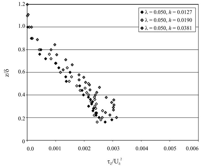
**Figure 5.** Height normalized by boundary layer depth ( $z/\delta$ ) plotted with normalized Reynolds shear stress ( $\tau_z/U_\delta^2$ ) of all element sizes for  $\lambda = 0.050$ .
