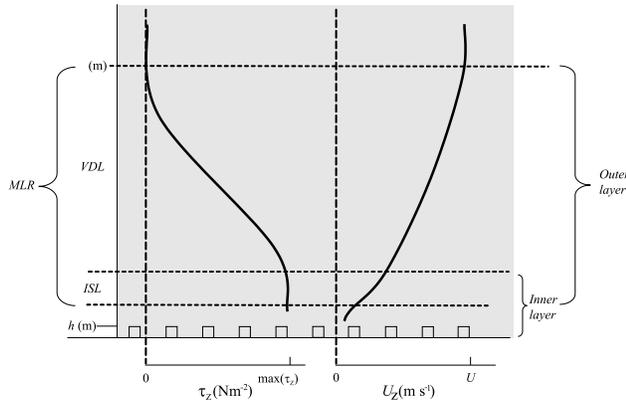
**Figure 1.** Schematic of a developed boundary layer ( $\delta$ ) over roughness elements of height,  $h$  (m). Plotted are interpretations of the Reynolds stress ( $\tau_z$ ) profile and velocity ( $U_z$ ) profile. Also labeled are the zones identified within the text of the inertial sublayer (*ISL*), maximum logarithmic layer (*MLR*), and outer-layer velocity-defect law (*VDL*).
