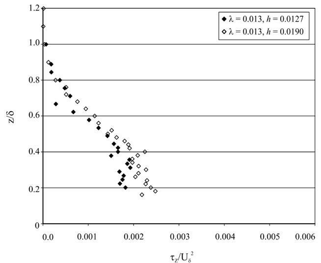
**Figure 6.** Height normalized by boundary layer depth ( $z/\delta$ ) plotted with normalized Reynolds shear stress ( $\tau_z/U_\delta^2$ ) of all element sizes for  $\lambda = 0.013$ .
