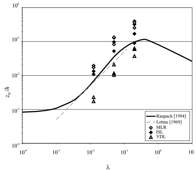
**Figure 11.** Roughness length normalized by element height ( $z_o/h$ ) plotted against  $\lambda$  calculated from the velocity profile fitted to the inertial sublayer ( $u_{*ISL}$ ) and the maximum logarithmic region ( $u_{*MLR}$ ), and the calculated  $z_o/h$  from the velocity-defect law (*VDL*). Also plotted are the models of *Lettau* [1969] and *Raupach* [1994].
