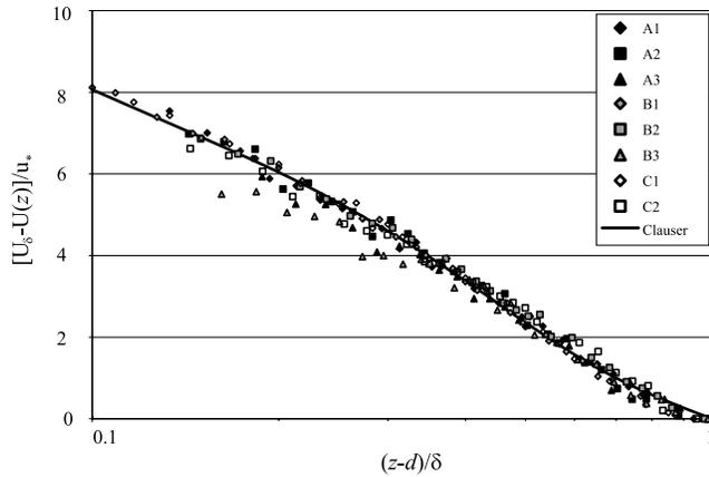
**Figure 3.** Mean velocity profiles plotted as outer-layer dimensionless form. The line is from the canonical profile model of *Clauser* [1956].
