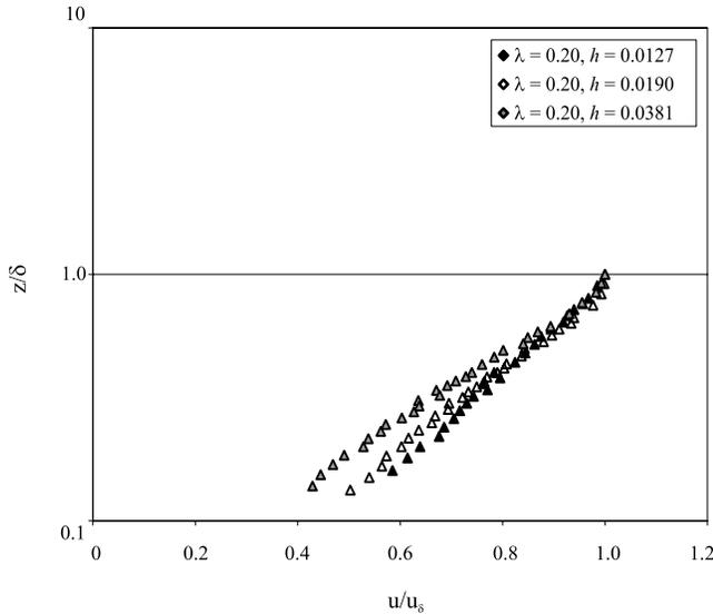
**Figure 7.** Height normalized by boundary layer depth ( $z/\delta$ ) plotted with velocity normalized with velocity at  $\delta$  for  $\lambda = 0.20$  for all cube sizes.
