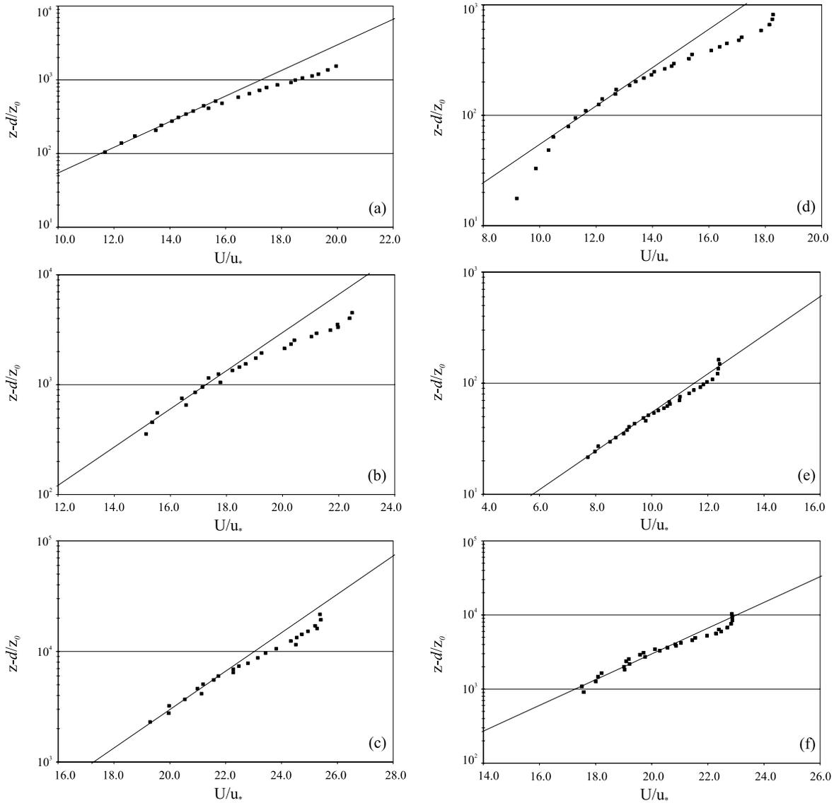
**Figure 8.** Logarithmic profile normalized height ( $z-d/z_0$ ) plotted with dimensionless velocity ( $U/u_*$ ) for the small cube at (a)  $\lambda = 0.01$ , (b)  $\lambda = 0.050$ , and (c)  $\lambda = 0.013$ , for the medium cube at (d)  $\lambda = 0.01$ , (e)  $\lambda = 0.050$ , and (f)  $\lambda = 0.013$ , and for the large cube at (g)  $\lambda = 0.20$  and (h)  $\lambda = 0.050$ . Solid line is the law-of-the-wall.
