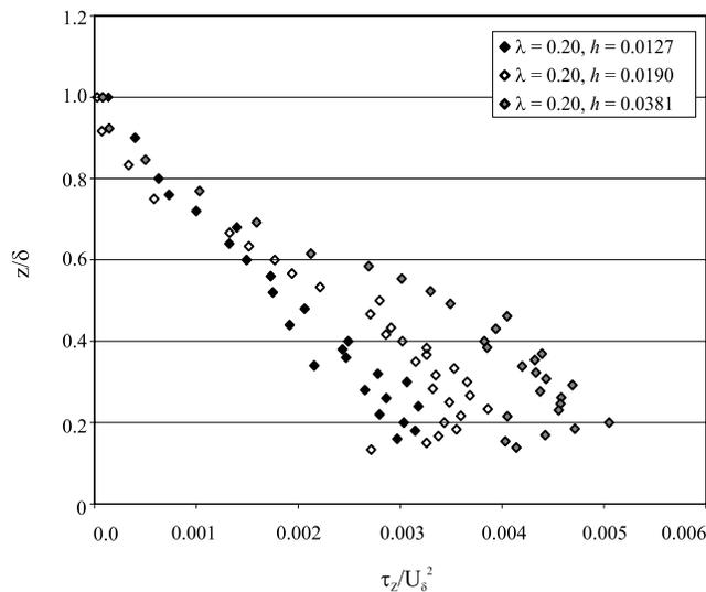
**Figure 4.** Height normalized by boundary layer depth ( $z/\delta$ ) plotted with normalized Reynolds shear stress ( $\tau_z/U_\delta^2$ ) of all element sizes for  $\lambda = 0.20$ .
