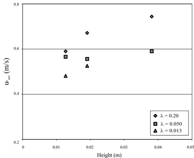
**Figure 9.** Shear velocity calculated from *HFA* within the *ISL* ( $u_{*uw}$ ) plotted against the cube size and grouped by  $\lambda$ .
