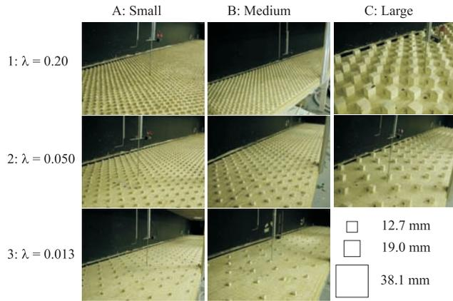
**Figure 2.** Photographs of the element configurations for all runs.
