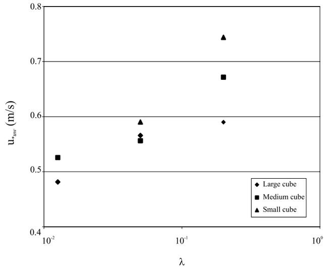
**Figure 10.** Shear velocity ( $u_{*uw}$ ) calculated from *HFA* plotted against  $\lambda$  grouped by cube size.
